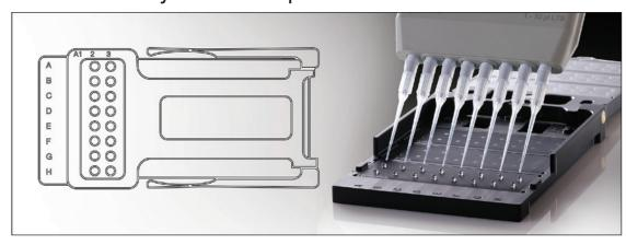
Turn your Cytation 5 into a micro-volume analysis system with Take 3. You can run 16 or 48 samples in one run to save a lot of time compared to single-sample devices. Gen5 is pre-programmed for ssDNA, dsDNA, RNA and protein quantification in 2 µL.
