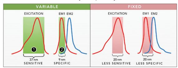
The plate reader optics of Cytation uses a quad monochromator design with variable bandwidth. The bandwidth can be set anywhere between 9 and 50 nm in 1 nm increment. Large bandwidth (1) settings provide increased sensitivity and lower limits of detection. Small bandwidth settings (2) provide increased specificity when multiple signals are present, which reduces signal crosstalk and enhances assay performance.
