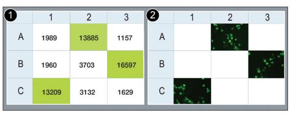
(1) Plate reader quickly identifies GFP positive wells. (2) Only GFP positive wells are imaged, saving both time and computer memory.
