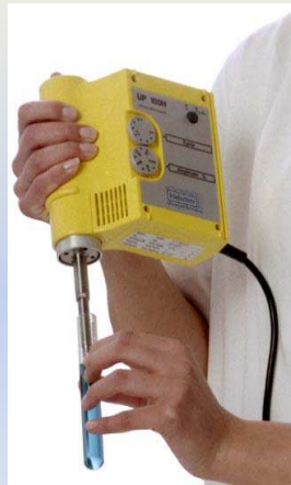
UP100H - compact light-weight ultrasonic device
