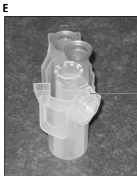
1.5 ml microcentrifuge tube lid is in the wrong slot of the rotor adapter
