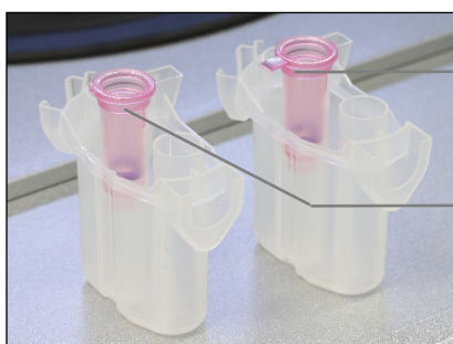
Comparing correct and incorrect removed column lids
