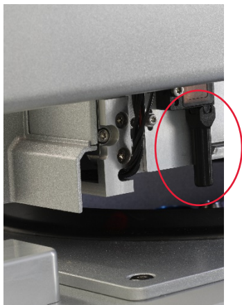
Black beam columnator (see red circle) of the ultrasonic sensor
