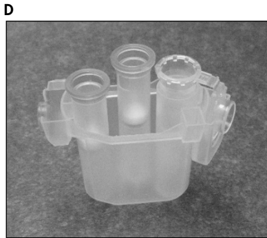
1.5 ml microcentrifuge tube lid not pushed down into slot
